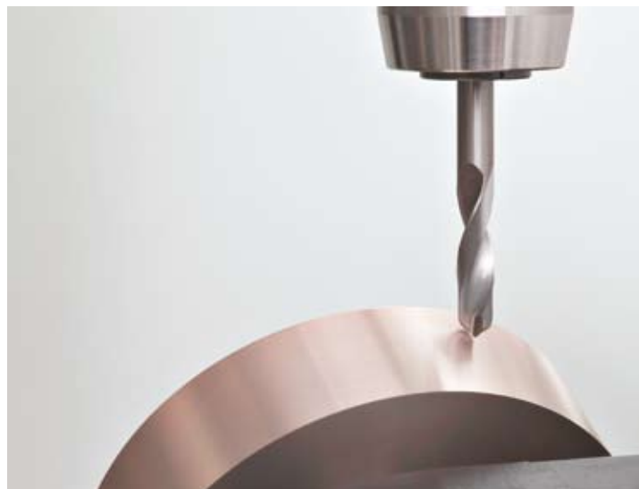
Eroding the plunge-in PCD-tip of a drill bit with the new software package - no problem!
