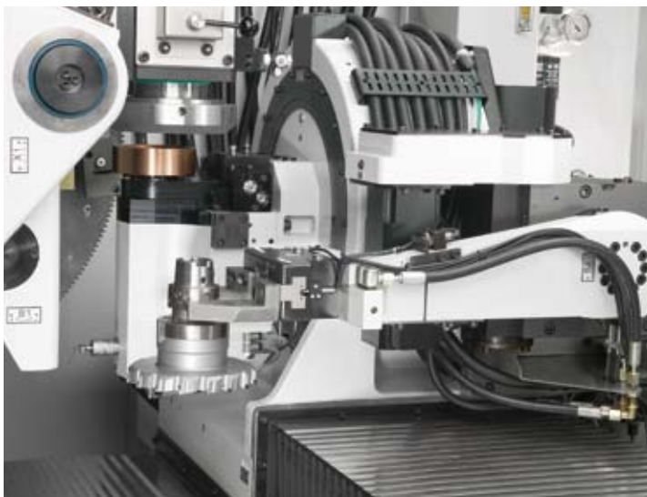
Reliable and efficient: Automation made by VOLLMER. Tool changing process of a PCD-tipped cutter.
