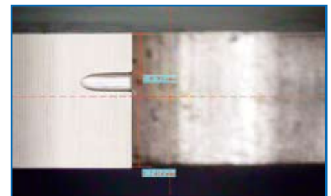
Inspection of chip breaker groove
